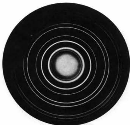
Fig. 1. Film AgBr polycristallin.
